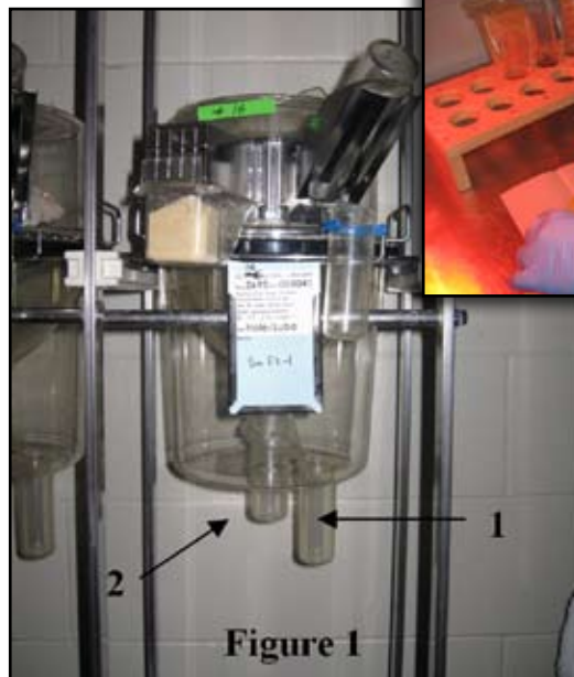
Figure 1: The rats are gavaged and housed in the metabolic cages for 72 hours (every 24 hours). Metabolic caging is necessary in order to distinguish the truly absorbed metal (gastro-intestinally absorbed, i.e., bioavailable) from the metal excreted from the body in the feces. Urine and fecal output are collected in a separate collection tubes, preventing urine (arrow 1) from washing over and entering the feces tube (arrow 2).
